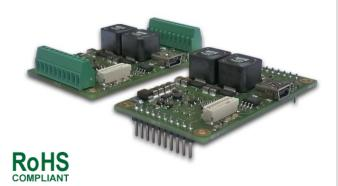
The TEC-1091 is a specialized TEC controller / power supply able to precision-drive a single Peltier element.
