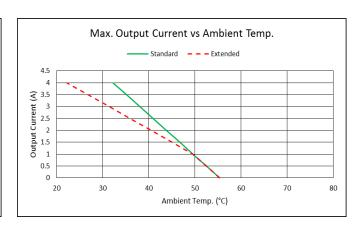
$\underline{\text{Standard}} \text{ or } \underline{\text{Extended}} \text{ Device Temperature Mode can be set as software setting.}$
