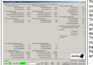
The included TEC Service Software is a powerful tool that allows monitoring, data logging and full configuration of the TEC-1089 via a standard USB or an RS485 connection from a PC running Windows.
