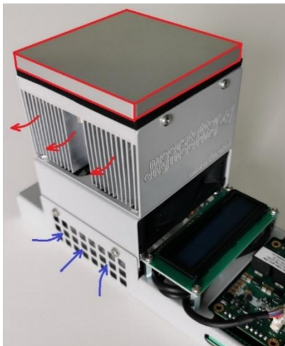
Figure 4: Hot/cold Plate of the SKT-1165
