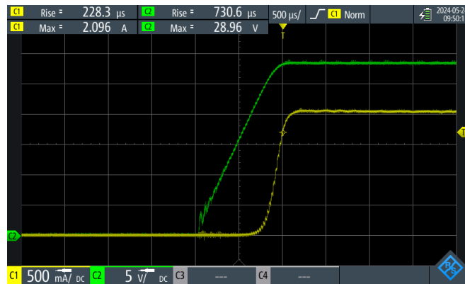
Figure 20. Tuned PID without slope limitation ( K_p=0.2 , T_i=0.000025 , T_d=0.00001 , Slope Limit= 10^{12} )
