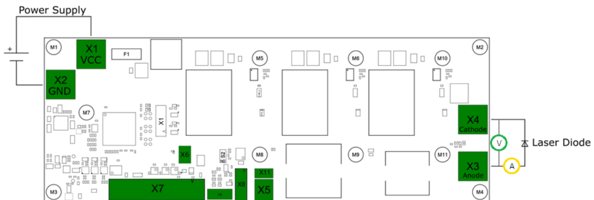
Figure 10. LDD-1303 setup with measurement probes on output yellow: CH1, green: CH2
