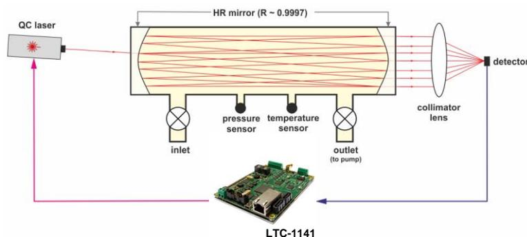
**Figure 2** Illustration of OA-ICOS. In AMICA, both laser diode control and detector signal acquisition and processing is done by the LTC-1141 as described below.
