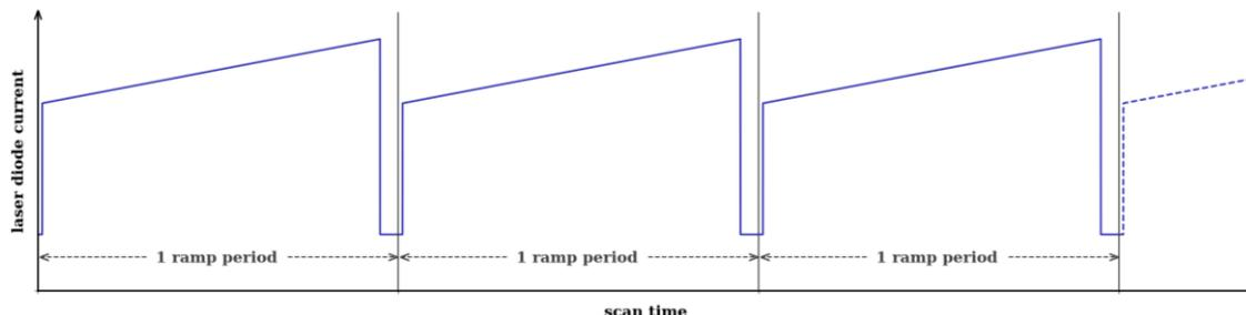
**Figure 3** Laser current modulation as typically applied in OA-ICOS.
