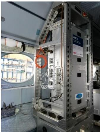
**Figure 1** Photograph of AMICA installed inside the cabin of the German research aircraft HALO
