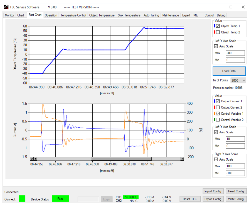
Figure 8. "Fast Chart" tab with panels for the object temperature (top) and output current / PID control variables (bottom).
