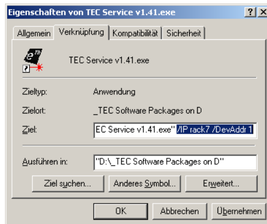
Figure 14. Creation of a customized link to a copy of TEC Service Software that will start up fully configured thanks to added application arguments.
