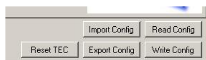
Figure 11. For reset-parameters to become activate, the unit needs to be power-cycled or reset by pressing 'Reset TEC' in the bottom right corner of the Service Software.
