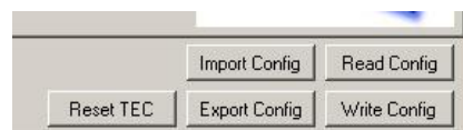
Figure 10. For reset-parameters to become activate, the unit needs to be power-cycled or reset by pressing 'Reset TEC' in the bottom right corner of the Service Software.
