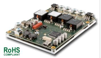
The TEC-1122 is a specialized TEC controller / power supply able to precision-drive two independent Peltier elements.
