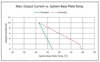
Test Condition: TEC Controller pressed with 1.2kPa to an aluminum System Base Plate without any thermal conductivity material in between. Using a good thermal conductivity material is recommended for high output currents. Standard or Extended Device Temperature Mode can be set as software setting.
