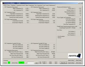
The included TEC Service Software is a powerful tool that allows monitoring, data logging and full configuration of the TEC-1089 via a standard USB or an RS485 connection from a PC running Windows.
